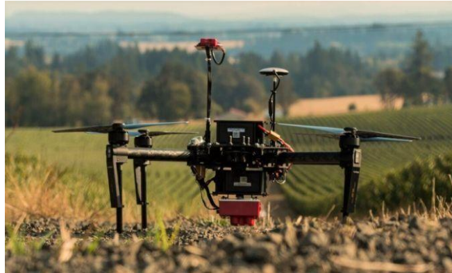
Fig.2.1. Remote sensing and imaging using drone
