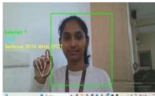
Figure 3. ASL-Based Sentence Formation Using Gesture Recognition
